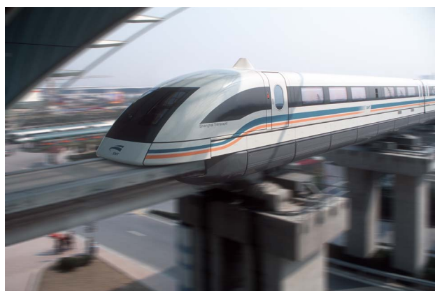
Fig. 13. Transrapid synchronous long-stator EMS system (Germany).
