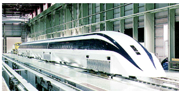
Fig. 12. Magnetic levitation U-shape synchronous long-stator EDS system (Japan) [12].
