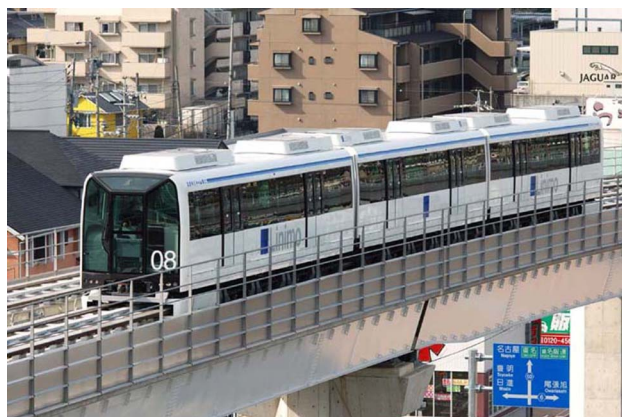
Fig. 11. Linimo short-stator LIM EMS system (Japan) [11].
